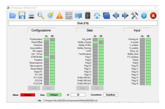
Once you have selected the desired bit configuration, you must send it to the converter using the **Out** button. The **In** key is used to read the configuration of the drive in case the automatic reading is disabled.
