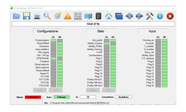
When the "**Positioner**" mode is selected, when the converter is switched on, the auxiliary digital input 2 is used as an end of stroke to search for the position of zero. The limit limit is considered reached when there are 0V for at least 100ms on the corresponding clamp. *No.B. Make sure that the bits in the configuration column for the Swap FC, FC1 CW, FC1 CCW, FC2 CCW fields are all zero.*
